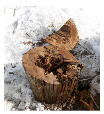
Extremely poor condition three pole deadend structure, left pole previously stubbed to provide support for weakened pole, right pole rejected due to excessive internal decay.
