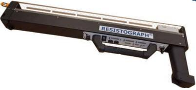
Using a long thin needle the electric power consumption of the resistograph drilling device is measured and recorded. The resistance data gathered provides a high linear correlation between the measured values and the density of the penetrated wood.
